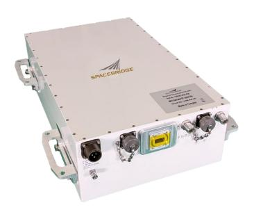
capability to utilize high MODCOD on small antennas for high data rate transmission. With an IP67 ingress protection rating, the device can be installed outdoor under the direct sun rays, at a short distance from the antenna feed, usually on the antenna boom, which contributes to significantly improve link budget and save electrical and maintenance costs.
