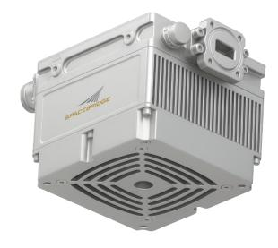
With an IP67 ingress protection rating, the device can be mounted outdoor under the direct sun rays on an antenna post/kingpost, on the platform behind the antenna, or inside the antenna hub, effectively eliminating the W/G RF loss commonly associated with indoor units. Additionally, it does not require airconditioning, resulting in significant reductions in ongoing electrical costs and maintenance expenses, while eliminating the need for nearby shelter construction
