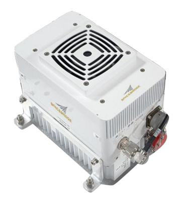
With an IP67 ingress protection rating, the device can be mounted outdoor under the direct sun rays on an antenna post/kingpost, on the platform behind the antenna, or inside the antenna hub, effectively eliminating the W/G RF loss commonly associated with indoor units. Additionally, it does not require airconditioning, resulting in significant reductions in ongoing electrical costs and maintenance expenses, while eliminating the need for nearby shelter construction
