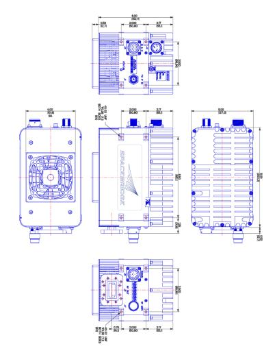
capability to utilize high MODCOD on small antennas for high data rate transmission. With an IP67 ingress protection rating, the device can be installed outdoor under the direct sun rays, at a short distance from the antenna feed, usually on the antenna boom, which contributes to significantly improve link budget and save electrical and maintenance costs.
