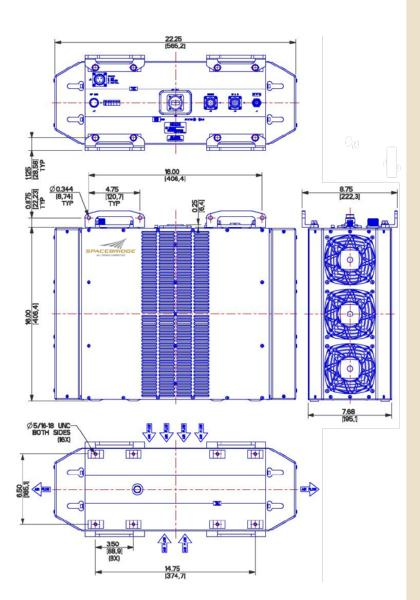
The device offers a wide range of monitoring and control capabilities, all easily accessible through Ethernet, serial RS232 and RS485 interfaces and Form-C dry contacts. It's the best-in-class solution for any demanding mobile or fixed application, designed for all-outdoor installations. This device does not require the additional air conditioning, or shelter. Therefore there is no W/G RF loss than installed in a shelter
